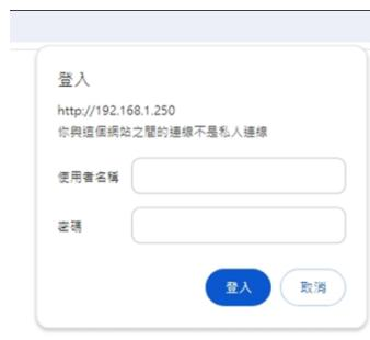
**Step 3:** Type IP address of SN-1 PLUS (192.168.1.250) in the web browser/ or Network Management Station (NMS) to connect to web-server/SNMP agent
